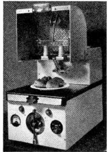
RADIO RE-HEATER. —Intended for re-heating pies, sausage rolls, muffins and other ready-cooked snacks (as opposed to cooking from the raw) this equipment, made by Radio Heaters, of Wokingham, works at R.F. on the dielectric heating principle. Power output, 0.5kW; frequency 75Mc/s.
